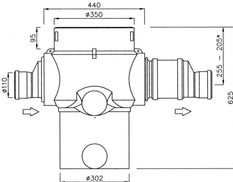
The connection to pipes DN110 can be carried out with customary KG pipe (2 reductions; 1 slip-on sleeve, see drawing on the left).
